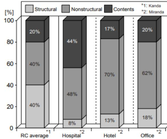
Figure 4. Repair Cost of Building Components after Seismic Event [6]
